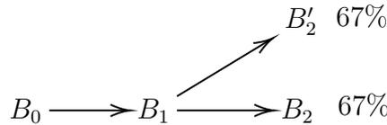
Figure 2: Finalizing a block requires a supermajority of 67%. Therefore, the chain can fork only if an attacker controls at least 67% of all stake and at least 34% of all stake is slashed.
