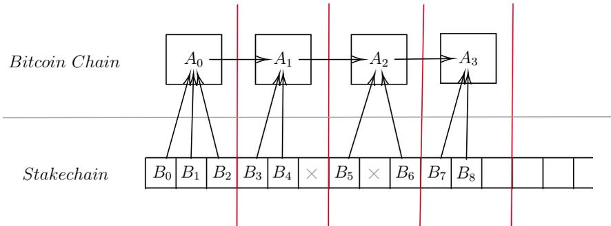
Figure 6: Sidechain blocks have to commit to bitcoin block hashes. The height of the bitcoin block must be at least the same height as in the preceding sideblock. In this example there are at most 3 sideblocks per mainblock. This ensures basic synchronicity.
